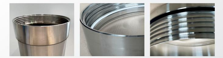
The specially developed GWE PureLine<sup>®</sup> aseptic well pipe connection, designed to be seamlessly free of gaps and dead space, is manufactured with the highest quality materials and finishes. The GWE PureLine<sup>®</sup> aseptic well pipe connection is fully ground, stained and passivated on the inside. Thanks to the minimized possibility of infiltration and the capacity to entirely remove residues, contamination with particles and germs is prevented from the very beginning.
